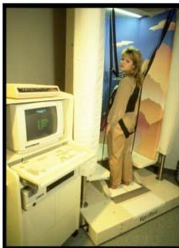
This test evaluates how well you are able to use the visual, vestibular and sensory systems during balance. The Sensory Organization Test (SOT) measures body sway under six different test conditions that are each completed three times. You will be tested with your eyes open and eyes closed, with the platform on which you are standing stationary or moving with your sway, and several combinations of these test conditions.
